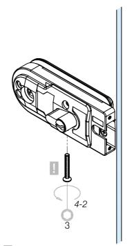
Screw length not longer than 35mm! (scope of supply)
